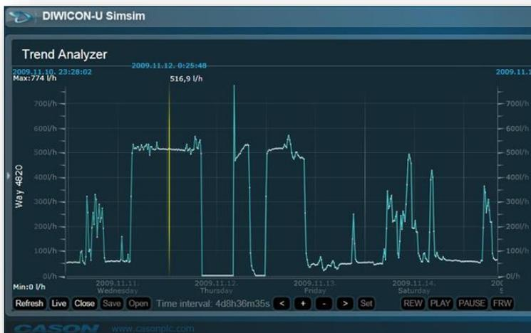
Anomalies can be easily detected observing consumer trends. **500 l/h continuous consumption** can be seen even during the night at this consumer. This can be caused by leaks and breaches in the water supply lines of the household.
