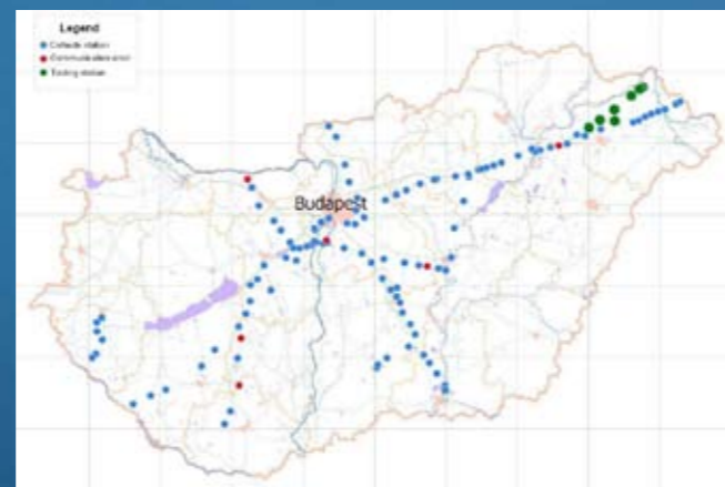
Online overview of the cathodic stations along the Hungarian oil and product pipeline network where DIWICON-K devices are installed
